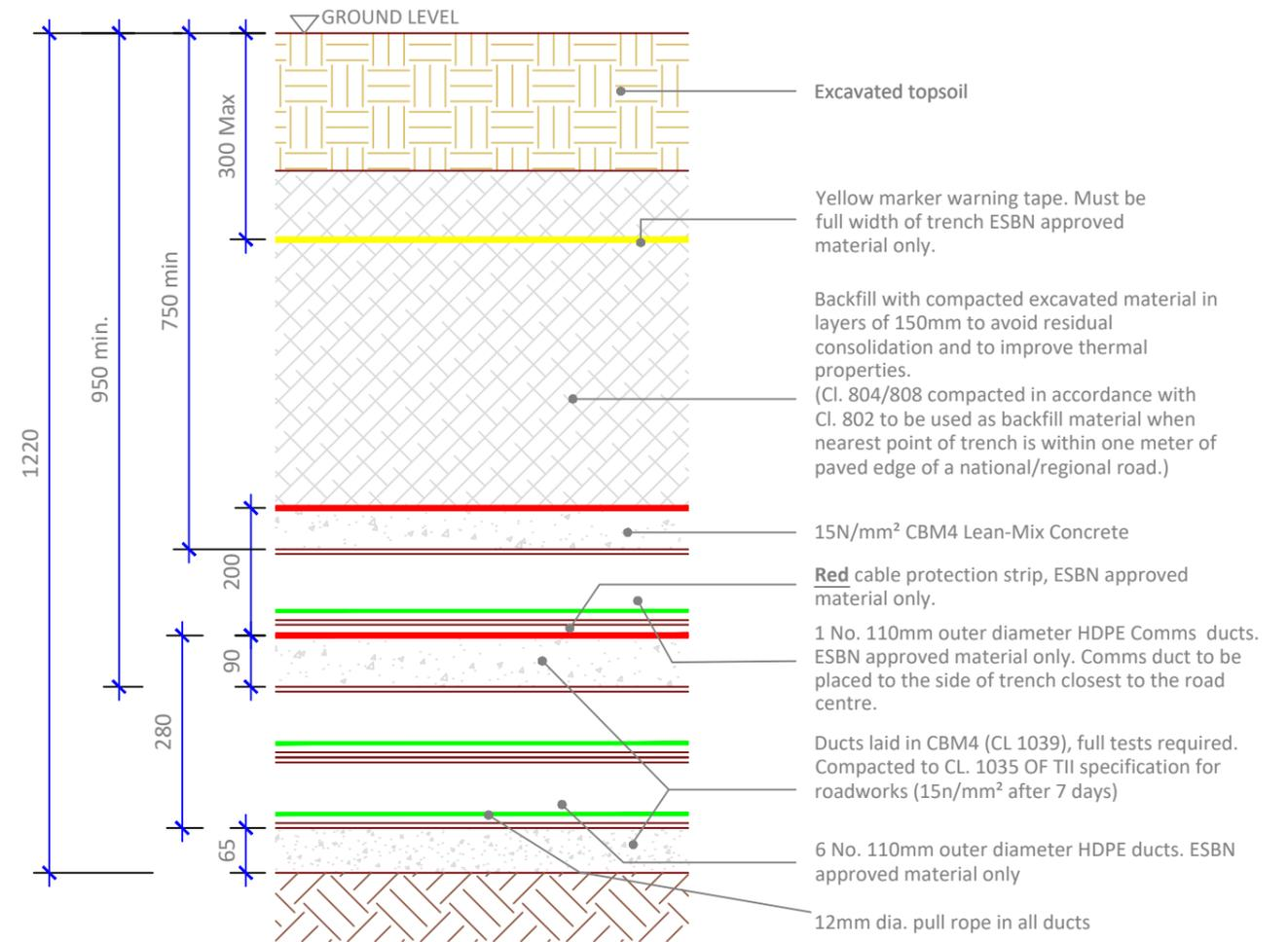
**Typical Elevation Through Off Road Sections**
